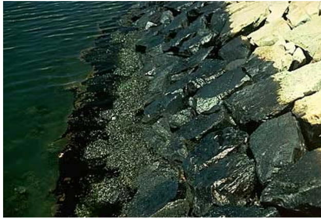
Figure 74: Coat Oil Thickness (Visible Oil <math><0.1\text{ cm}</math> that can be Scraped with Fingernail)
