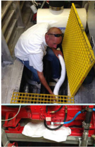
Figure 44: Oil Absorbent Materials to Catch Leaks on Board Recreational Boats 141
